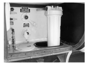
Insert the new filter cartridge, positioning it so the opening in
